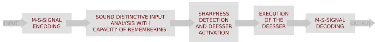
Figure 30: Block diagramm of the Weiss De-Esser plugin
