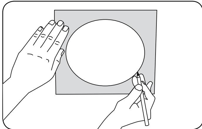
**ENG** Now hollow out an appropriate installation opening in the wall/ceiling. When laying loudspeaker cable from amplifier to installation point, be sure that the cable ends about 30 cm (12") beyond the wall cutout.
