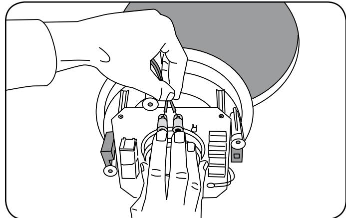
**ENG** If the red mounting tabs are in a horizontal position and the screws firmly screwed in they are ready for installation.
