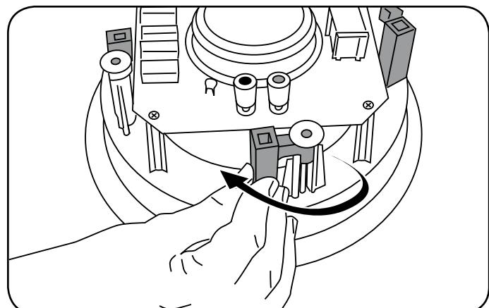
**ENG** Place the loudspeaker system in the installation hole and tighten the screws, so that the speaker is fixed in the installation opening. Important: To prevent damage to the mounting tab, do not twist screws too tightly.
