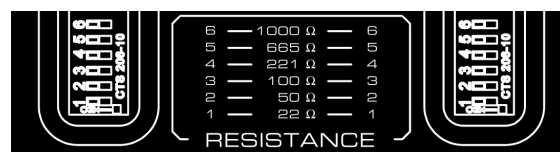
Figure 3: Left and right channel DIP switches for resistance loading adjustments
