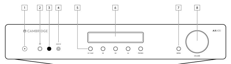
1. Power button - Switches the unit between Standby mode (indicated by dim LED) and On (indicated by bright LED). Standby mode is a low power mode where the power consumption is less than 0.5 Watts.
