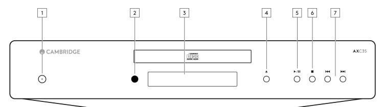
**1. Power button** - Switches the unit between Standby mode (indicated by dim power LED) and On (indicated by bright power LED). Standby mode is a low power mode where the power consumption is less than 0.5 Watts. This product has APD (Auto Power Down) enabled as default. After inactivity of 20 minutes, the product will automatically switch to Standby.
