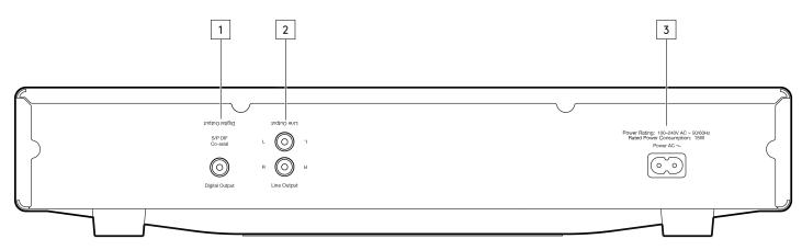
**1.** S/P DIF CO-AXIAL DIGITAL OUTPUT (AXC35 ONLY) - For input to a separate DAC or digital recording machine. To obtain best results, use a high quality 75 Ohm digital RCA interconnect cable (not one designed for normal audio use).
