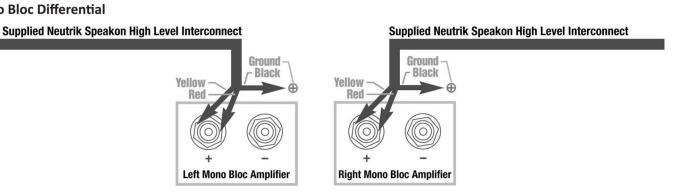
• If connecting a single REL as a dedicated centre channel sub, an insider tip is to consider connecting to the rear of the speaker, rather than routing the REL High Level enable all the way back to the amplifier. Connect the black wire of the REL to the negative centre channel speaker terminal; twist together the red and yellow wires and connect this paired cable (red/yellow paired together) to the positive centre channel speaker terminal.
