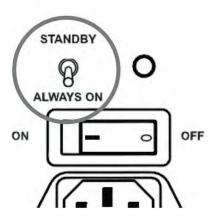
During initial setup, use the REL this way. After initial setup, if you wish to employ the standby mode, simply move the power mode switch into the up position to "STANDBY".
