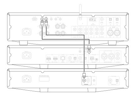
**Note:** The CXA, CXN and CXC all have an Auto Power Down (APD) function. If APD is enabled and one of the devices is switched on but inactive, the device will automatically power down after the selected APD time. This will then switch off all the other connected devices, due to the Control Bus connection.
