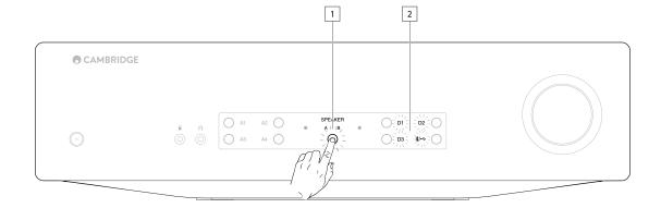
Note: Press the Speaker A/B button once to leave the Setup menu and place the CXA back into Standby mode.
