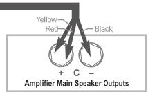
• If connecting a REL as a dedicated rear channel sub, connect the black wire of the REL to either the left rear or right rear negative speaker terminal; connect the yellow wire to the left rear positive speaker terminal; connect the red wire to the right rear positive speaker terminal. If the amplifier is of balanced differential design, please follow the instructions in the section above labeled Differential Connection.
