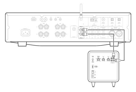
2. If you are using a receiver, or amplifier with a dedicated sub out then connect the Minx X301 using the left channel (LFE/Sub) input.
