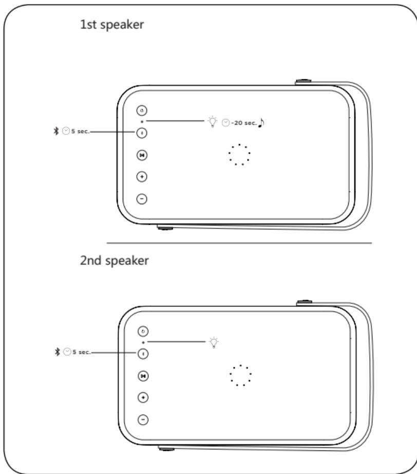
**EN** Beolit 20 can be stereo paired either in the Bang & Olufsen app or manually. To set this up manually, press and hold the Bluetooth button on the first speaker for 5 seconds until the indicator turns white. Wait for 20 seconds until an audible prompt is heard, and then perform the same operation on the second Beolit 20. Both devices will then make an audible prompt to indicate that they are connected.
