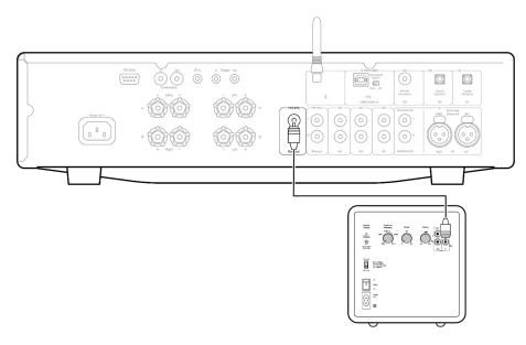
3. Once connected you can decide where to position your subwoofer. As low frequency content is largely unidirectional, you can experiment to find a place that suits your setup.
