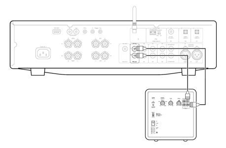
2. If you are using a receiver, or amplifier with a dedicated sub out then connect the Minx X201 using the left channel (LFE/Sub) input.
